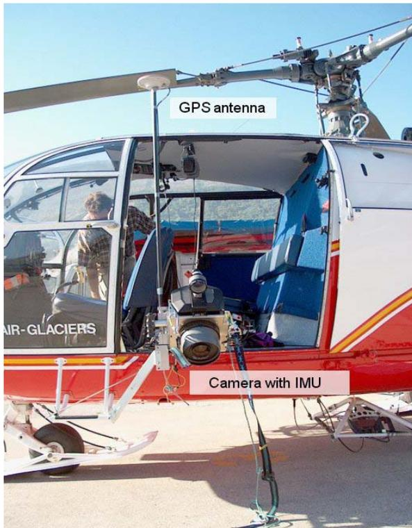
Fig. 3 : Tomtecs camera mounted with GPS antenna. The INS is mounted under the camera. During the picture session, the block camera-antenna is only hold by the operator.
