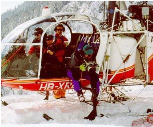
Fig. 5: The camera is held and the vibrations are damped by the body of the operator.
